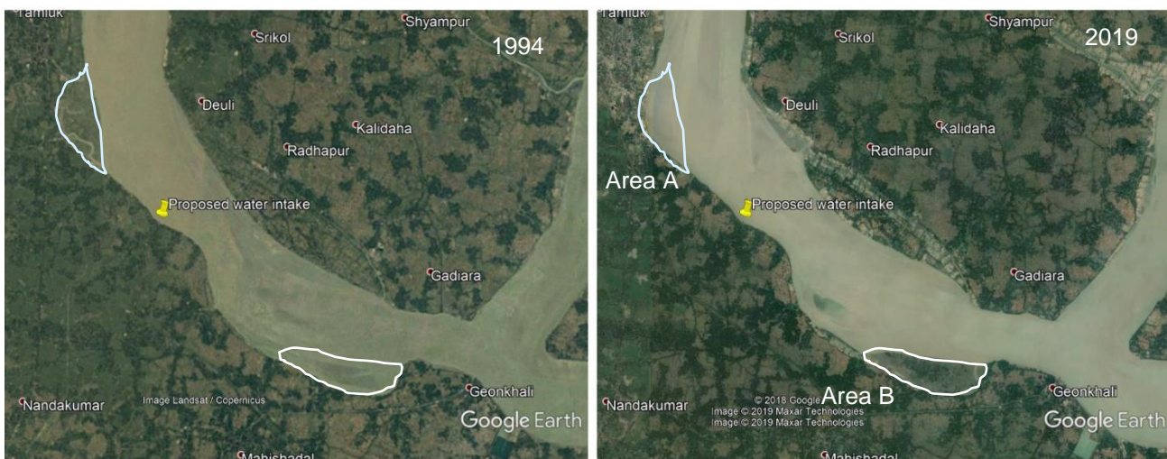
Figure 5-4 Two possible sites for area reclamation for reservoirs. Area A (near Tamluk, today submerged) is 230 ha, area B (North of Mahishadal-Geonkhali Road, today mudflats) is 270 ha. The left figure shows a satellite image from 1994, the right is from 2019.
